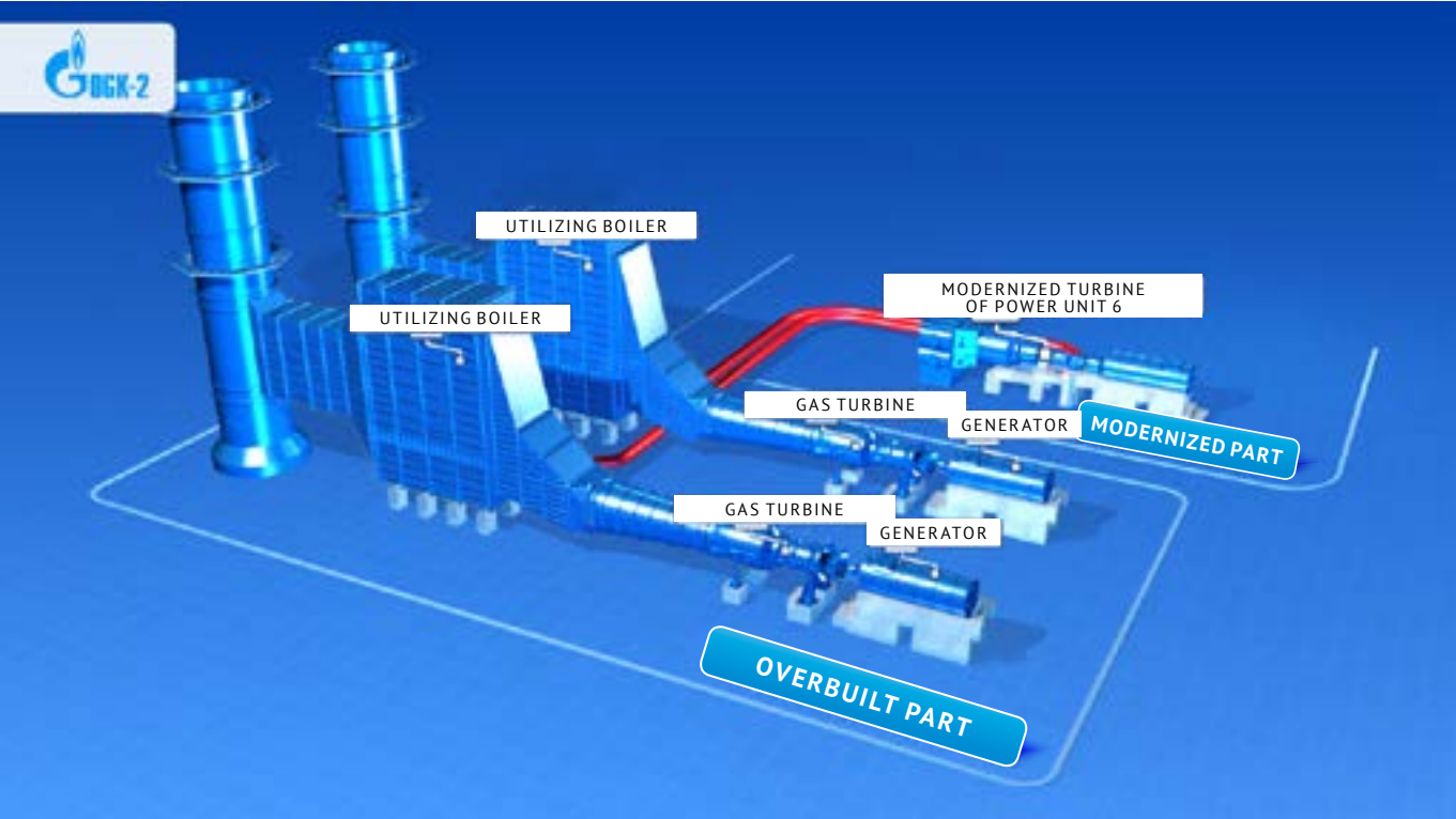
Schematic diagram of the CCGTU-800 combined cycle gas turbine unit at Kirishskaya GRES
